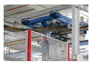
BU: Wide variety of solutions for factory and logistics automation: Conductor rail system 0815 in an Electrified Monorail System
